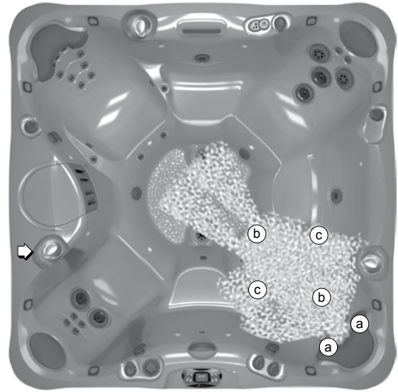
JET PUMP 1 – JET SYSTEM 2
